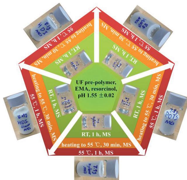
Figure 1. Versatile preparation methods and appearances of various liquid cores and MCs: UF, EMA, and MS denote urea-formaldehyde, poly(ethylene- alt -maleic anhydride), and mechanical stirring, respectively.
